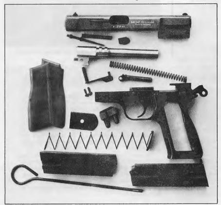
is more evidence of hand-fitting on the PJK-9HP. Its 13-round staggered-column magazine with gray plastic follower remains as difficult to load as the FN original.
